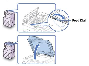
8 While using the feed dial to turn the resin roller, wipe the resin roller and its surroundings with a water-moistened cloth. Then, wipe the area with a soft, dry cloth.
